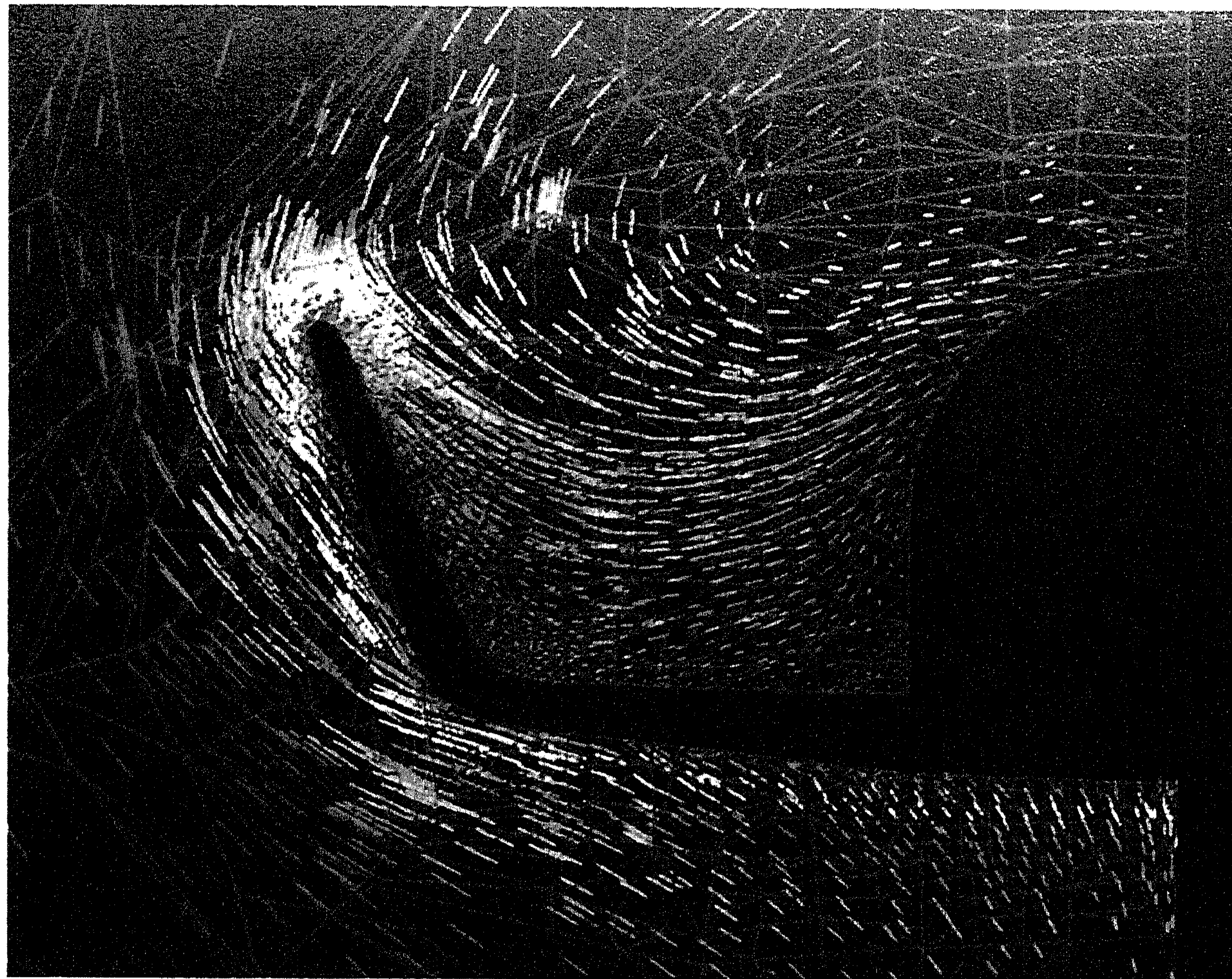
Figure 2. Streamline distribution around a half cross-section of the Hermes spaceplane. Applying multigrid methods, CWI studied numerical solutions of equations describing the flow around heavier-than-air craft as a part of the European space programme. Photo: Dassault.
